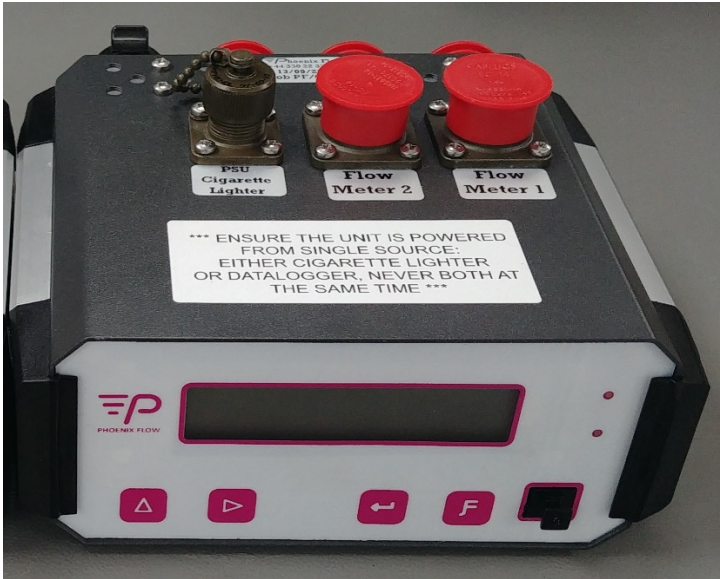
Figure 3: Custom Aluminium Enclosure with Mil-Spec connectors
